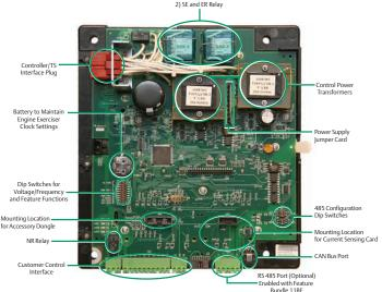
Fig. 8: ASCO SERIES 300 Microprocessor Controller
