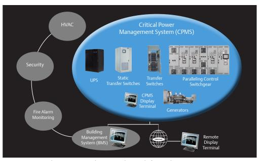
PowerQuest provides monitoring, alarming and control of Critical Power Management Systems, which comprise transfer switches, paralleling control switchgear, gensets, circuit breakers, UPS, loadbanks, distribution and other gear. It also integrates with building management systems.
