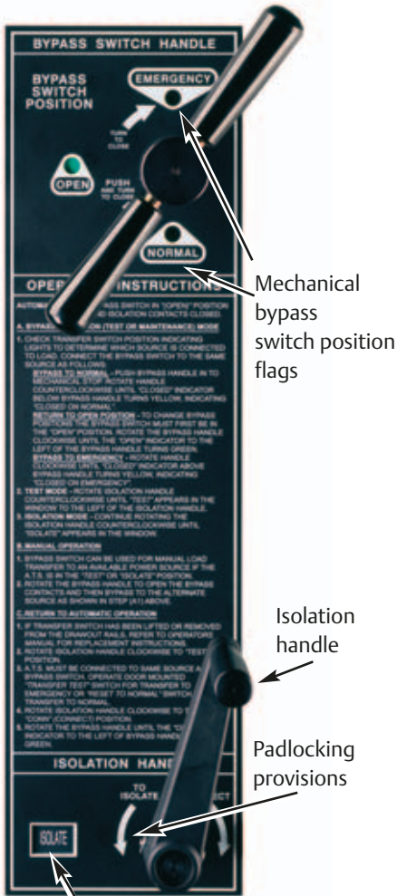
Fig. 12: Bypass-Isolation Switch user interface
