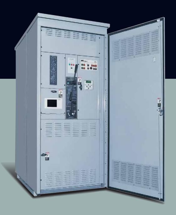
ASCO 7000 SERIES Soft Load Power Transfer Switch with bypassisolation, rated 2000 amps in a Type 3R outdoor enclosure The ASCO 7000 SERIES Closed-Transition Soft Load Power Transfer Switch with bypass-isolation switching allows the switch to be inspected, tested and maintained without interrupting power, whether it's being provided from the utility or onsite generator.
