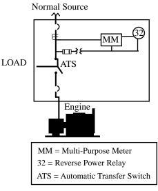
Fig. 8 One line diagram of the two source automatic transfer system shown in figure 7.
