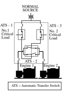
Fig. 12 One line diagram of the three source priority system shown in figure 11.
