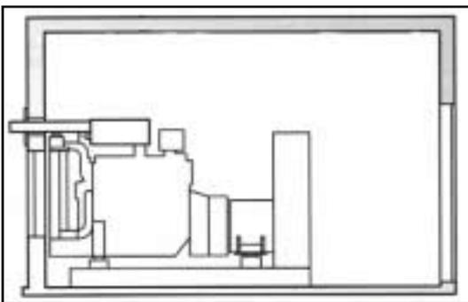
The exhaust pipe should be properly suspended, brackets must not be mounted on the generating set (except for original assemblies). An exhaust expansion coupling should be fitted on the engine outlet. The pipe diameter should never be smaller than the generating set exhaust outlet (please consult us for lengths longer than 6 m).
