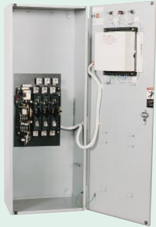
Fig. 8 Automatic Transfer Switch rated 3 pole 400 amperes with microprocessor controls on door.
