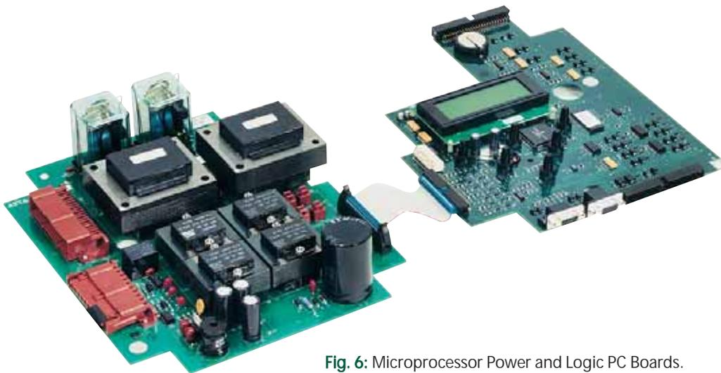
**Fig. 6:** Microprocessor Power and Logic PC Boards.
