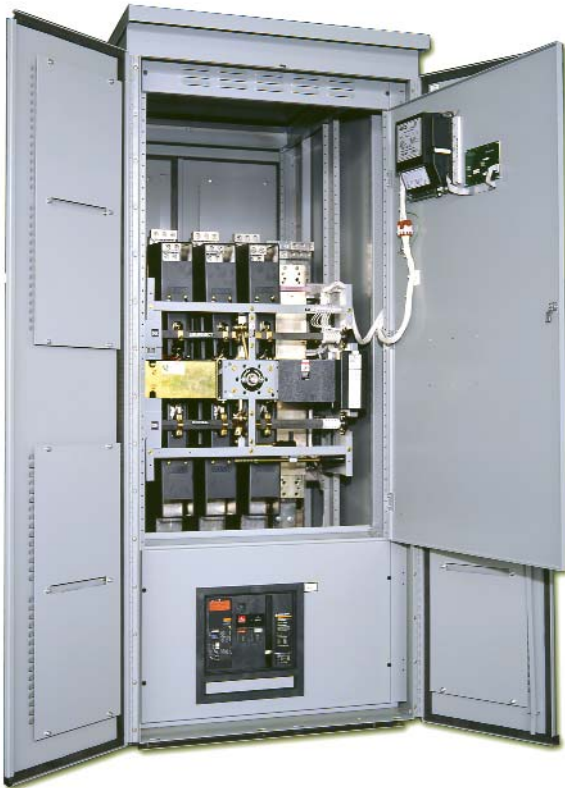
Fig. 15: ASCO Service Entrance Power Transfer Switch rated 3 Pole 2000 amperes shown in Type 3R secured double door enclosure with solid neutral
