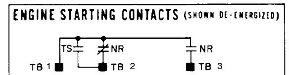
Figure 1-1. Engine starting contact label and location for 150–800 & 3000–4000 amp switches.
