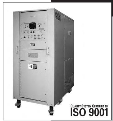
he Avtron Patriot Load Bank is a portable, self-contained unit that simulates electrical loads. It is ideal for routine load testing of standby diesel generating systems at remote sites or for factory production line testing of (UPS) Uninterruptible Power Supplies, turbines, or engine generator sets. This model provides resistive loading up to 700 KW at either 240/480 Volts AC in a convenient, and easy-to-use package.
