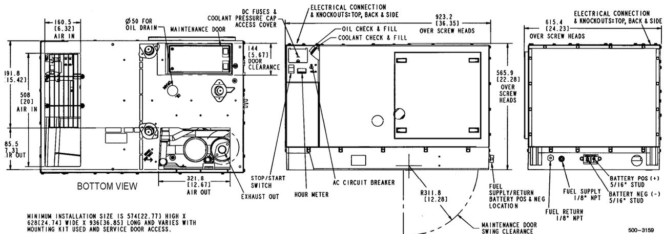
**Note:** This outline drawing is provided for general reference only and is not intended for design or installation. For more information see Operation and Installation manuals or obtain drawing 500-3159 and wiring diagram from your distributor/dealer.
