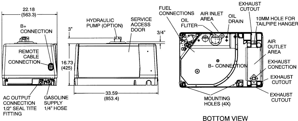
**Note:** This outline drawing is provided for general reference only and is not intended for design or installation. For more information see Operation and Installation manuals or obtain drawing 500-3349 and wiring diagram from your distributor/dealer.
