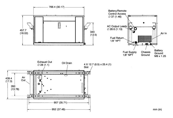
**Note:** This outline drawing is provided for general reference only and is not intended for design or installation. For more information see Operation and Installation manuals or obtain 500-4709 drawing and wiring diagram from your distributor/dealer.
