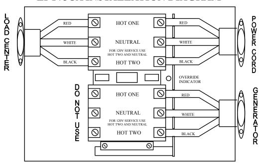
**CONTACTORS:** 3 Pole N.O. 240VAC, 75 Amps/Pole
