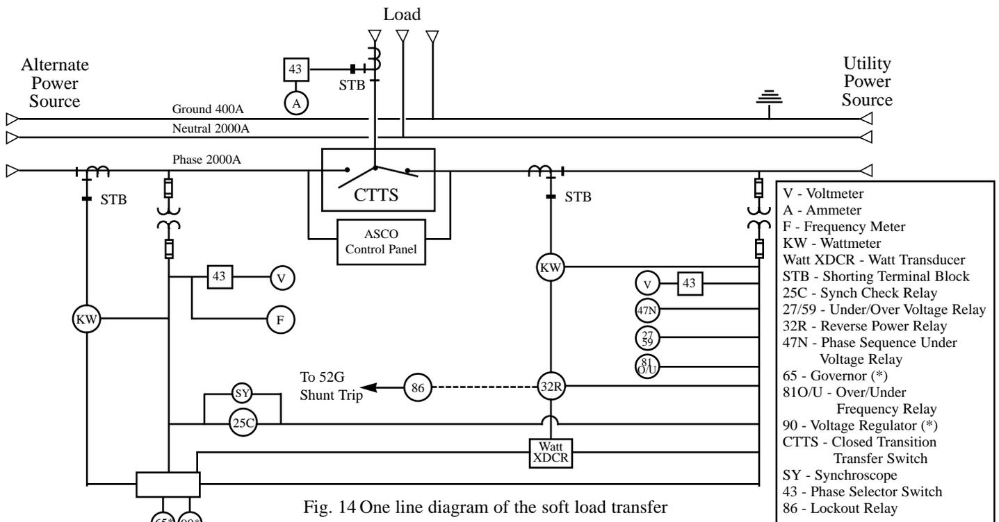
Fig. 14 One line diagram of the soft load transfer system shown in figure 13.
