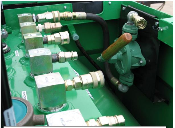
Note – The standard tank set up is 1 X 1" feed, 1 X ½" feed and 1 X ½ " return. The tank shown on the picture is modified to suit a particular application.
