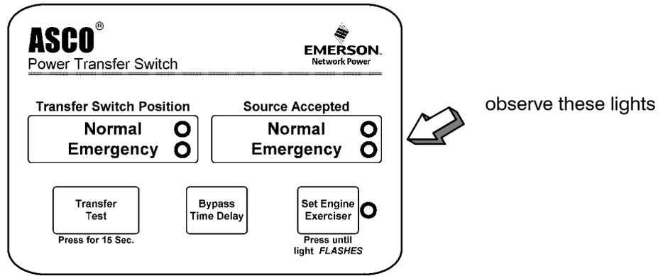
Figure 1-5. Standard controls and indicators.
