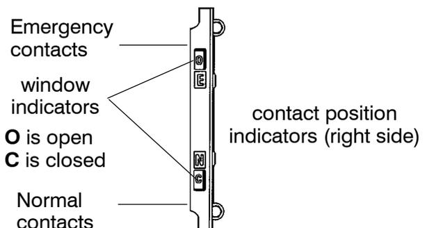
Figure 1-4. Maintenance handle operation and contact position indicators.
