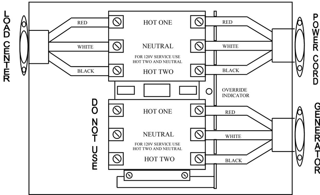
**CONTACTORS:** 3 Pole N.O. 240VAC, 75 Amps/Pole
