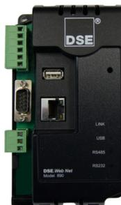
Further expansion is available by adding the optional "WebNet" gateway interface module. This device will allow comprehensive monitoring of the generator via the cloud including identification, location, and status. Some advantages of this module include: reduced site visits and maintenance costs • remote fuel management • fault analysis • asset tracking • automatic system alerts • maximized system up-time.
