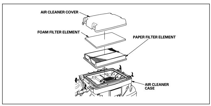
FIGURE 3-2. AIR FILTER ELEMENT AND WRAPPER
