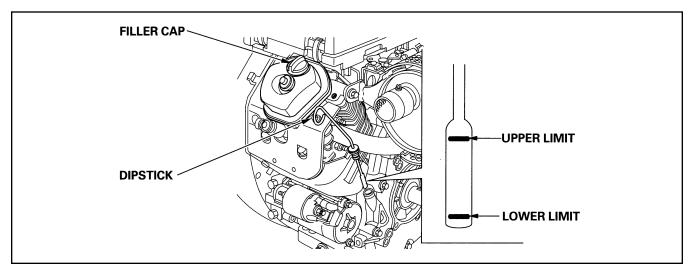
FIGURE 3-1. OIL LEVEL CHECK
